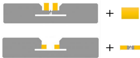
Figure 2: BitID tags enabled by shorting the IC (top) and separating the IC with the antenna (bottom)
